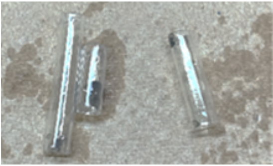
Figure 6. Photo of the tubing from Competitor A after 1 week soaking in VCAP.
