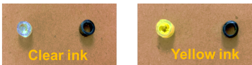
Figure 3. Left: cross-sectional area of the tubing after filled with clear ink and irradiated with a UV curing lamp. Right: cross-sectional area of the tubing after filled with yellow ink and irradiated with a UV lamp.
